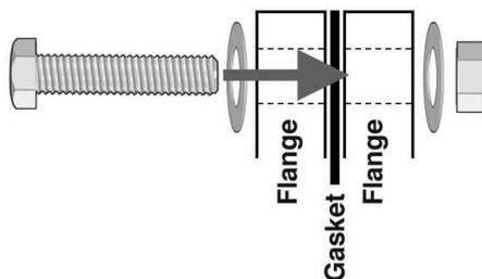
If using a compatible antiseize lubricant as recommended, apply the lubricant evenly with a brush directly to the bolt threads, and to the nut if desired. Cover the bolt from its tip to the maximum extent to which the nut will be threaded.
