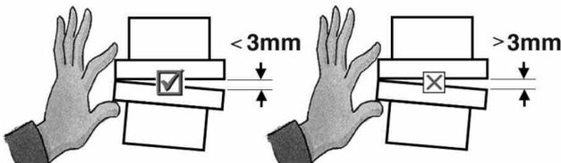
If the gap between the components cannot be closed by pinching them with one hand, or if the angle between them is too large, refit the system with proper alignment before bolting.
